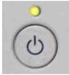
Fig. 2.3 Power switch on the front panel of 4051
